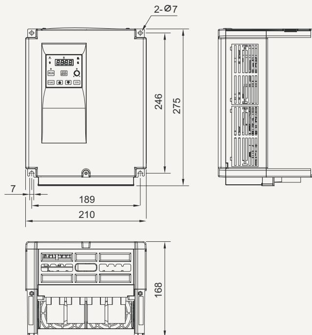
N700E-150LF/150HF, N700E-185LF/185HF, N700E-220LF/220HF
